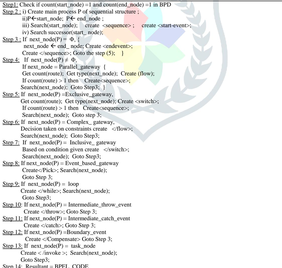
Figure 4. Mapping Algorithm BPMN To BPEL
