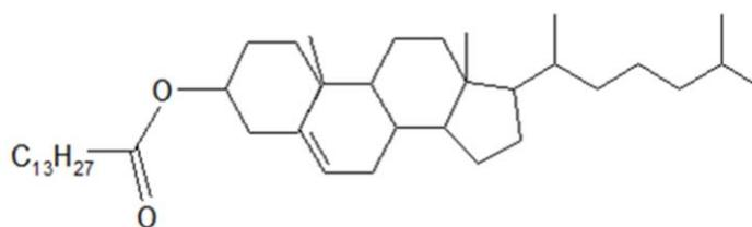
**Crystal (70.6 °C) SmA (78.6 °C) N\* (84.0 °C) Isotropic**
