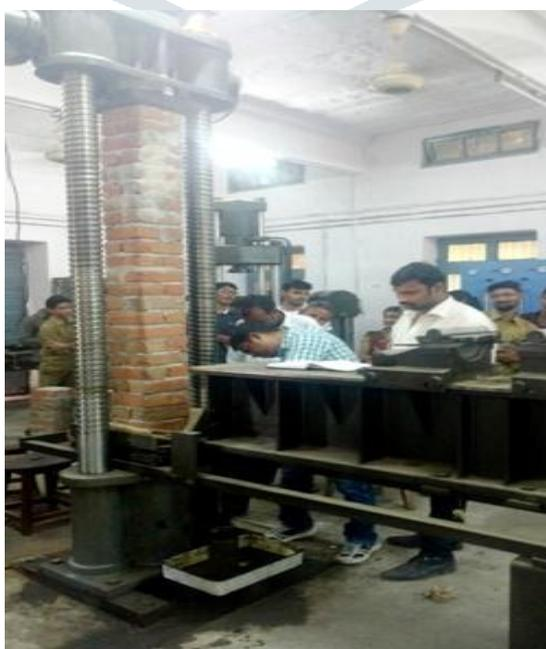
**Figure 2 Preparations for Test with Universal Testing Machine**
