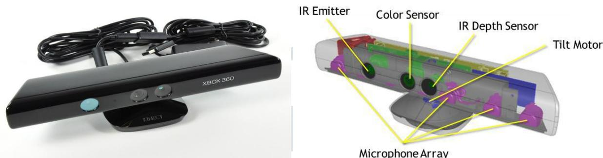
Figure 1 Kinect (XBOX 360) for Windows Sensor Components
