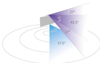
Figure 2 Kinect for Windows sensor field of view [9]
