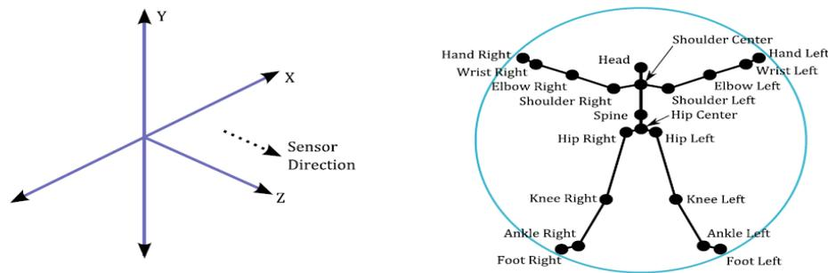
Figure 5 An illustration of the skeleton space. Figure 6 Tracked skeleton joints overview
