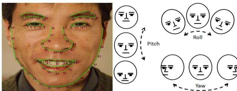
Figure 8 Tracked face points.[9] Figure 9 Head pose angles.[9]
