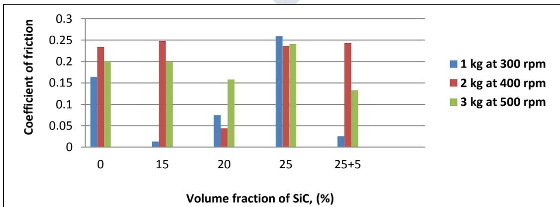
Figure 10: Shows change in coefficient of friction of AZ91 with different volume fraction of SiC and Al<sub>2</sub>O<sub>3</sub>
