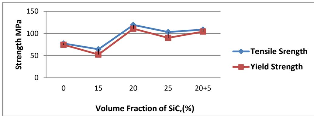
Figure 6: Change in yielding and tensile strength of AZ91 alloy as a function of volume fraction of SiC
