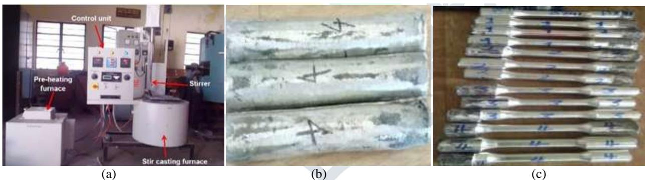
**Figure 1: (a) Stir casting setup (b) composite material after casting (c) prepared specimens for tensile test**
