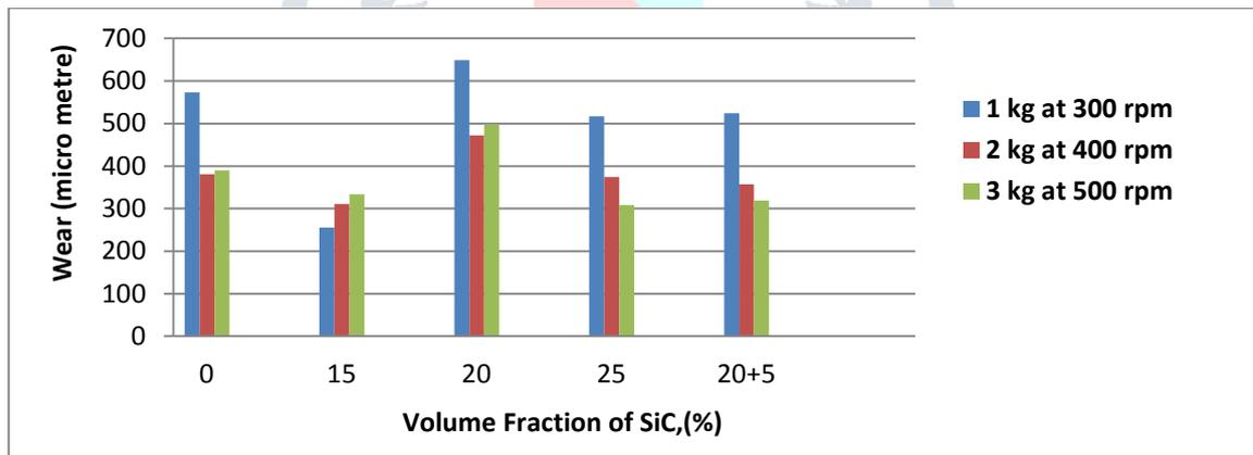
Figure 9: Shows change in wear of AZ91 as a function of volume fraction of SiC and Al<sub>2</sub>O<sub>3</sub>
