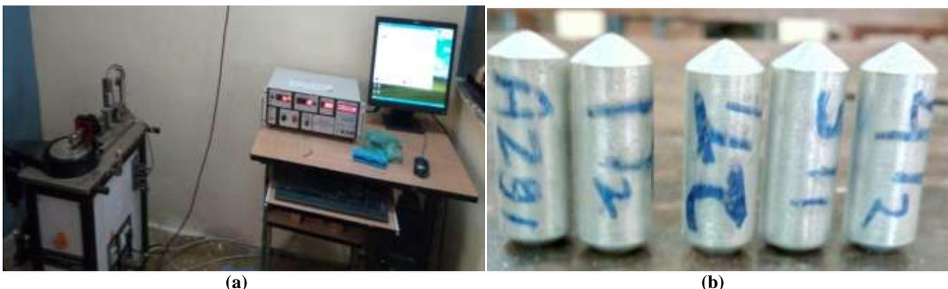
Figure 4: (a) Pin-on-disc wear test machine setup (b) prepared specimens for wear test of length 32 mm and dia 10 mm
