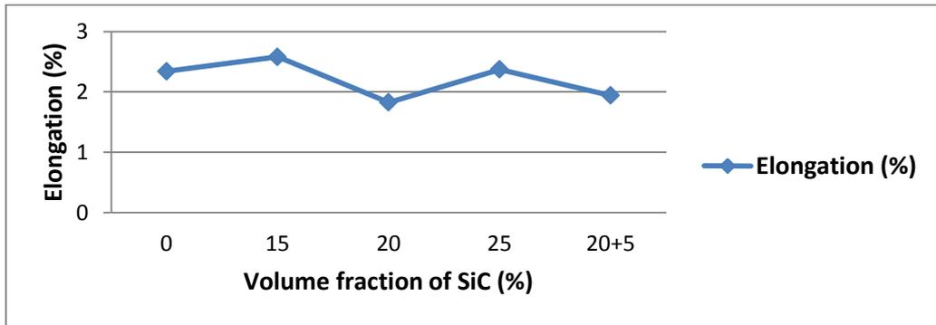
Figure 7: Variation of tensile elongation of AZ91 alloy with volume fraction of SiC
