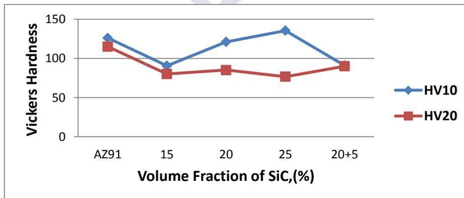
Figure 8: Variation of the hardness values of AZ91 with different volume fraction of SiC-particles
