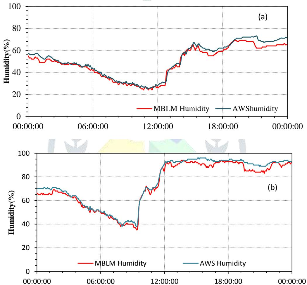
Fig. 7: Mini-Boundary Layer Mast (MBLM) and Portable –AWS observations.
