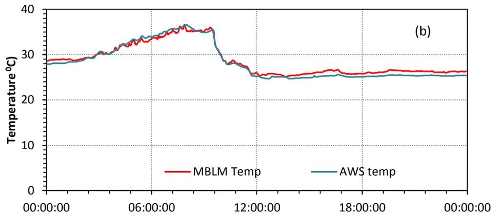
Fig.6: Evaluation of performance of the Portable–Automatic Weather Station (AWS) using Mini-Boundary Layer Mast (MBLM) observations (a) Diurnal variation of temperature observed on clear sunny day (20 April 2009). (b) Diurnal variation of Temperature observed on passage of thunderstorm precipitating clouds on 22 April 2009.
