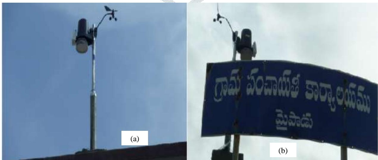
Figure 5: (a) AWS at Inagaluru (14°33.17N, 78°16.15E), ThondurMandal, YSR (Kadapa) Dist (b) AWS at Mypadu (14°30.36N, 80°10.36E), Indukurupeta, Sri Potti Sriramulu Nellore District
