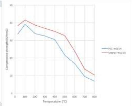
Fig 5: Variation of compressive strength with temperature for water quenched cube specimens exposed for 3 hours
