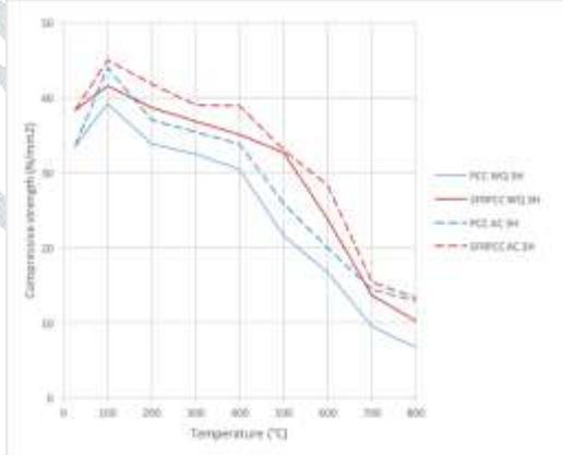
Fig 6: Variation of compressive strength with temperature for air cooled and water quenched cube specimens exposed for 3 hours
