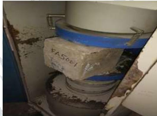
Fig 3 Placing of cube specimen in compressive testing machine
