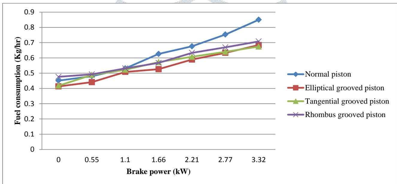
Fig.7 Fuel consumption vs Brake power
