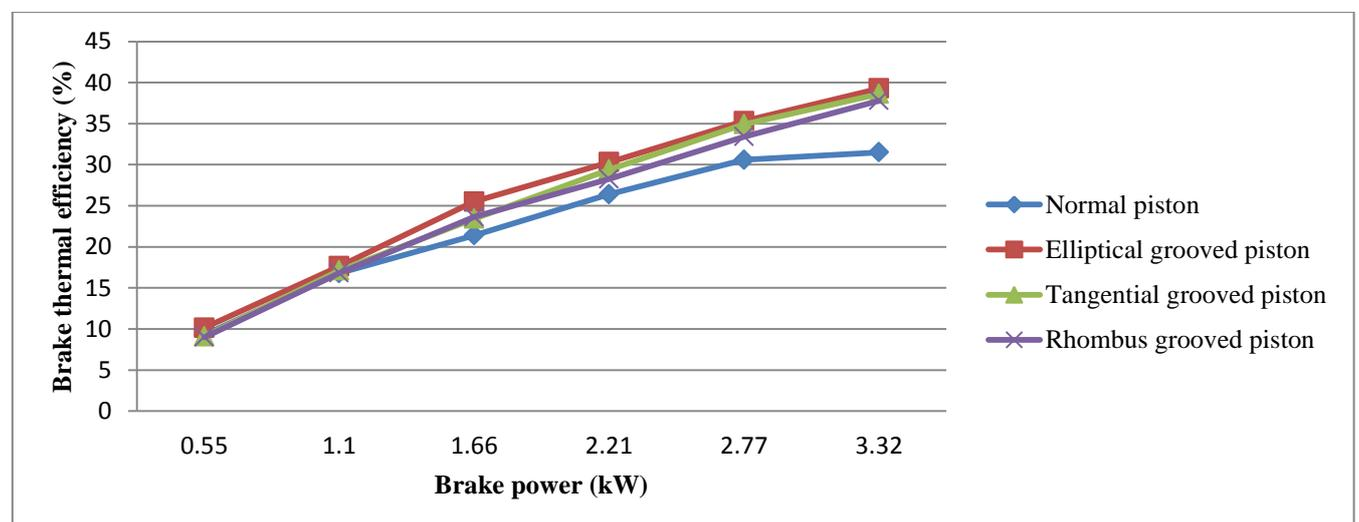
Fig.5 Brake thermal efficiency vs Brake power
