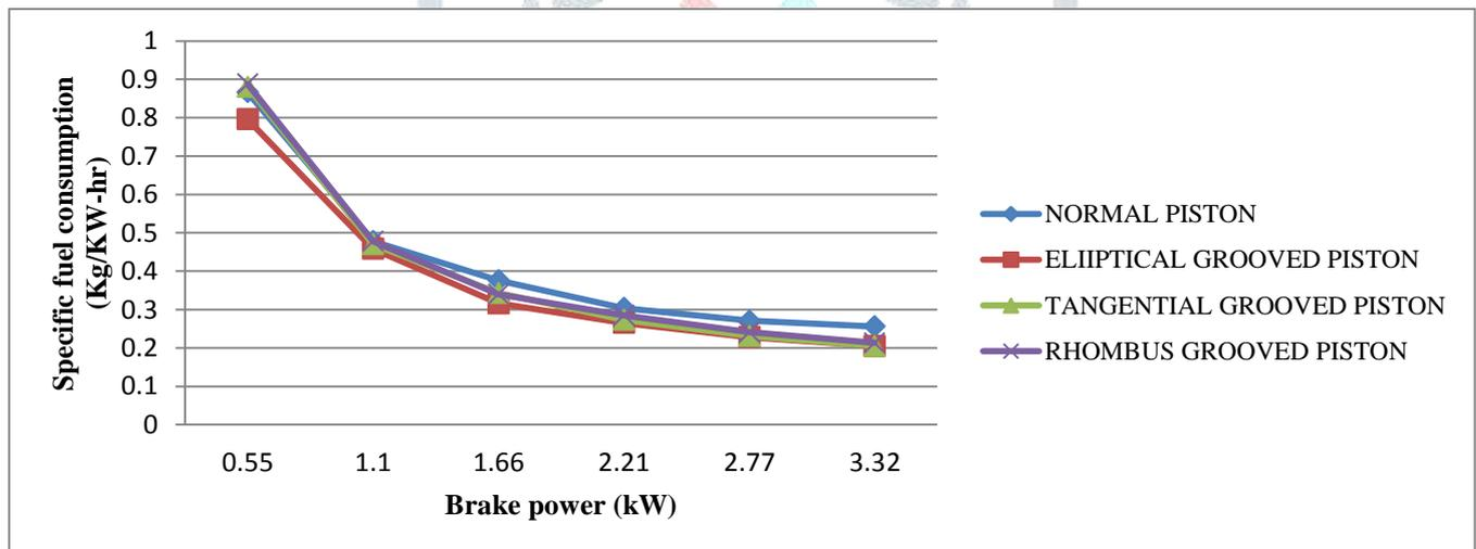
Fig.4 Specific fuel consumption vs Brake power
