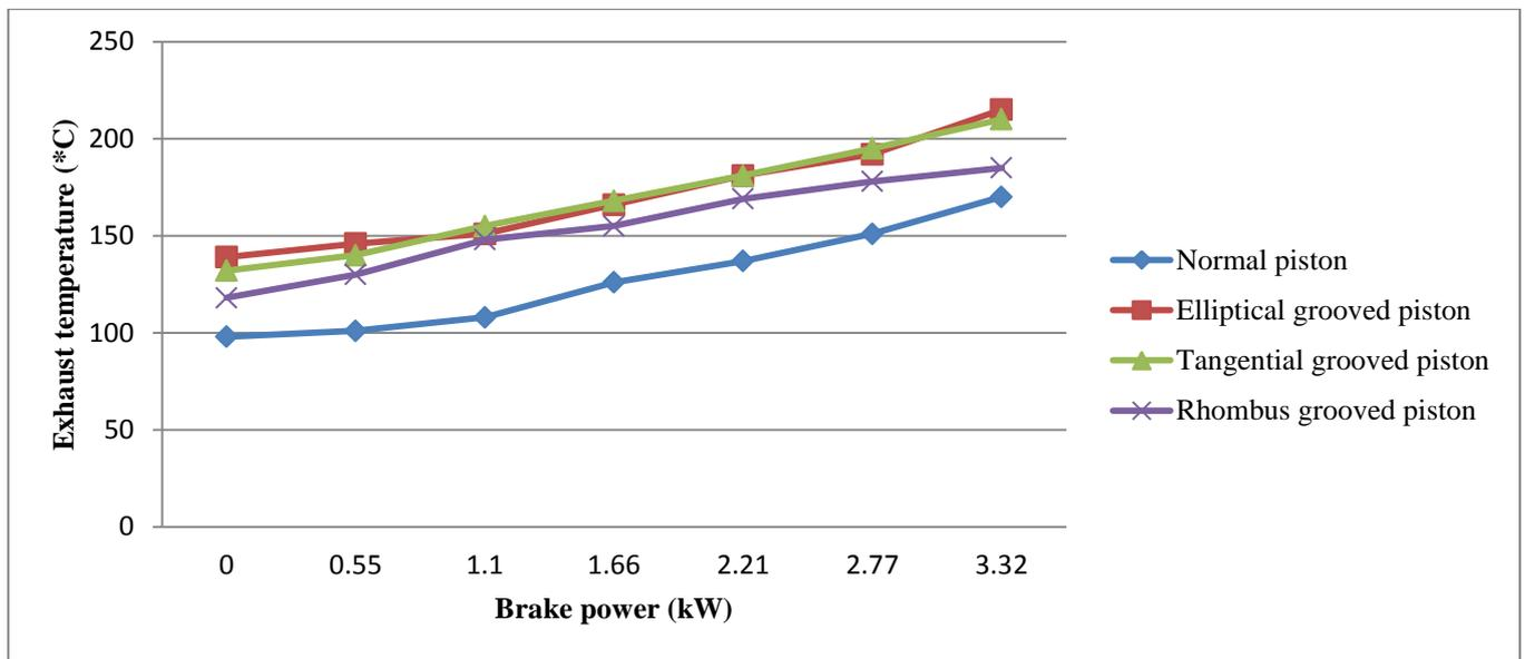
Fig.6 Exhaust temperature vs Brake power
