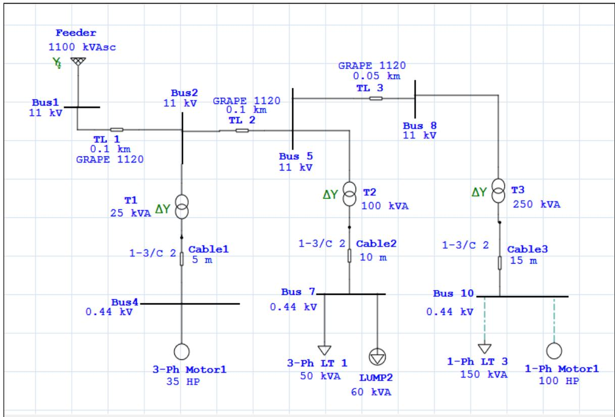
Figure.1 One line diagram of partial (up to node 3) 11KV town Feeder of HRECS using ETAP
