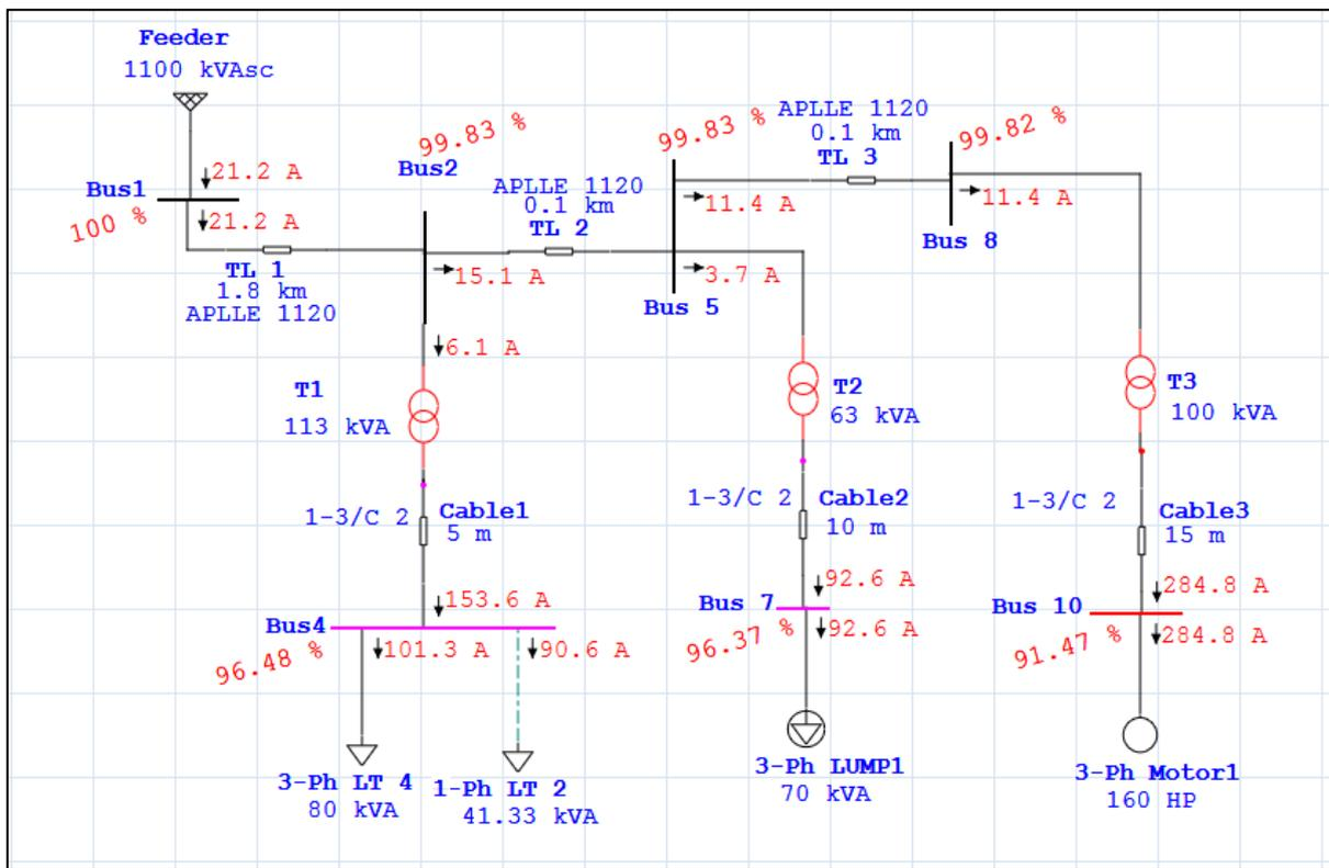
Fig 4. Load Flow Analysis of partial (up to node 3)11KV HESCOM IP Feeder using ETAP tool.
