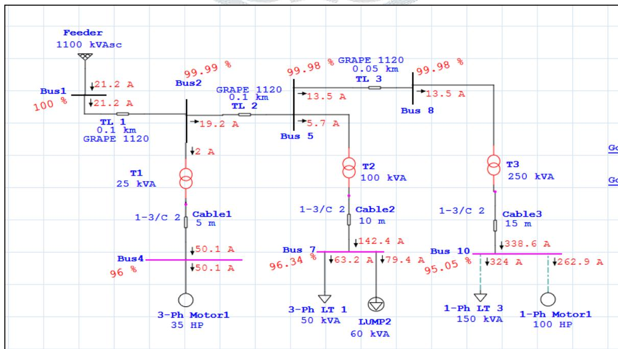
Figure.2 Load Flow Analysis of partial (up to node 3) 11KV town Feeder of HRECS using ETAP tool.
