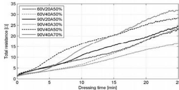
Fig. No. 1 Resistance vs Dressing Time at Speed of 10 m/s [9]
