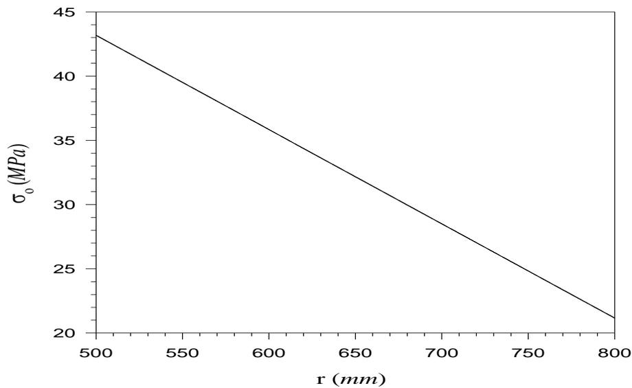
Fig. 2: Variation of Threshold stress with radius.
