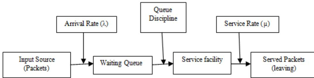
Fig. 1 Components of a basic queuing system
