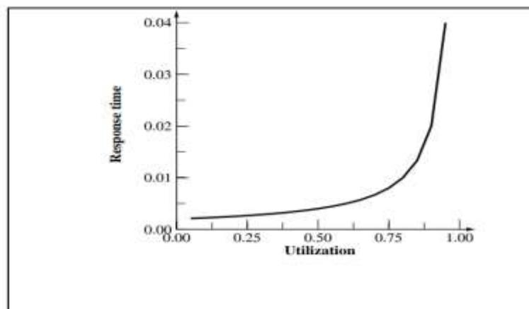
**Fig. 3: Graph between Utilization and Response Time of the Node**
