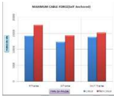
Figure 6. Nonlinearity effect on cable force
