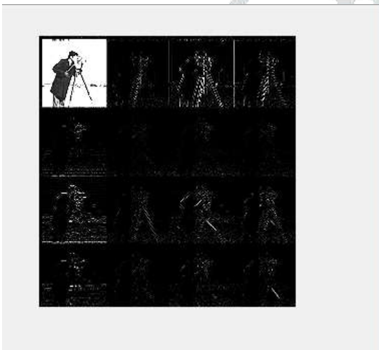
Figure 10 shows the compressed image of Cameraman after applying 3 rd haar discrete wavelet transform.
