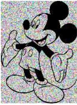
Fig. (xv) When mean filter is used for Poisson noise, PSNR: 11.7043 SNR: 9.0761 MSE: 4391.891
