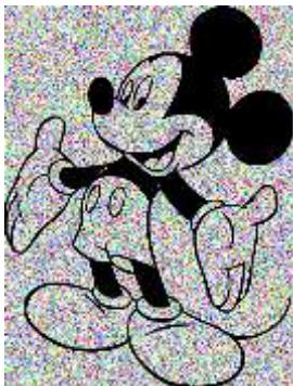
Fig. (xix) When mean filter is used for Speckle noise, PSNR: 11.7200 SNR: 9.0958 MSE: 4316.0000
