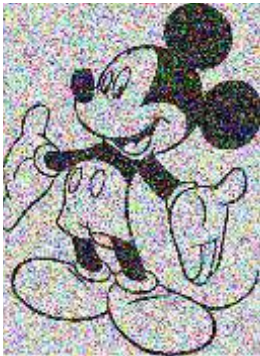
Fig. (xi) When mean filter is used for Gaussian noise PSNR: 11.7875 SNR: 9.6093 MSE: 4038.5261
