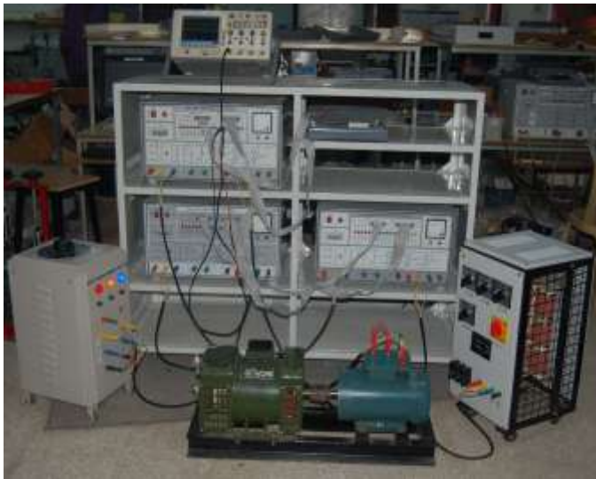
Fig. 12: Schematic of the experimental setup of matrix converter interfaced PMSG for wind energy conversion system
