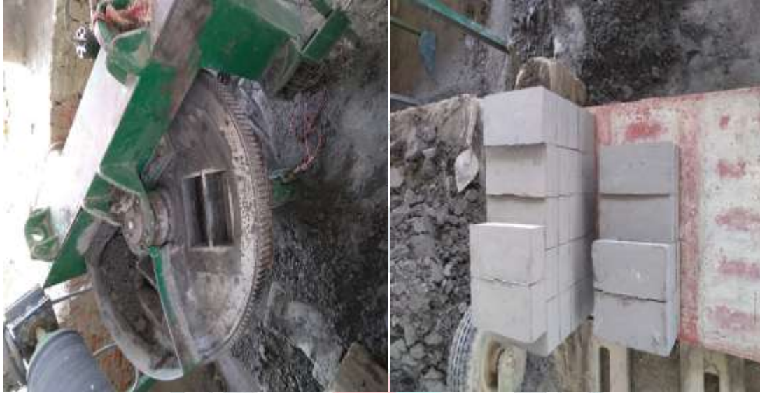
Figure 1: machine setup and fly ash bricks
