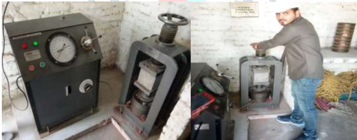
Figure 1: Compressive strength Test Machine and Testing of Cubes
