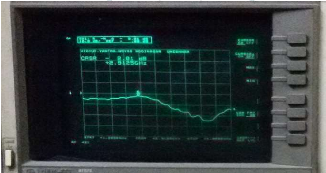
Figure 6: Response of third order stepped impedance micro-strip low pass filter (insertion loss) using network analyzer
