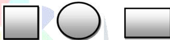
Figure 1.2: Section of concrete filled steel columns.
