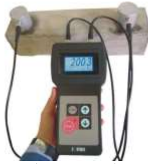
Fig.2 Ultrasonic Pulse Velocity test of cubes
