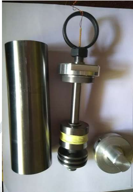
Fig 6: Manufactured MR Damper
