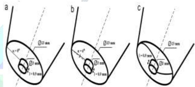
Figure 6: (a) Flat (b) conical concave and (c) scrolled shouldered tools [19]
