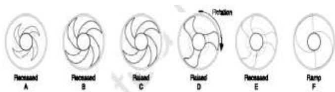
Figure 7: Schematic diagram of the six-unique tool shoulder geometry [23]
