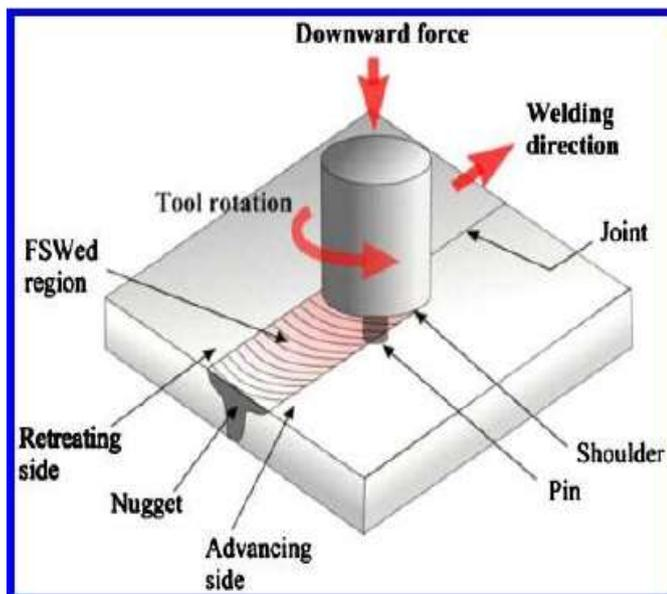
Figure 1: Principal of Friction Stir Welding <sup>[1]</sup>
