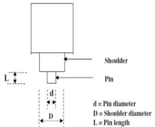
Figure 2: FSW Tool <sup>[2]</sup>
