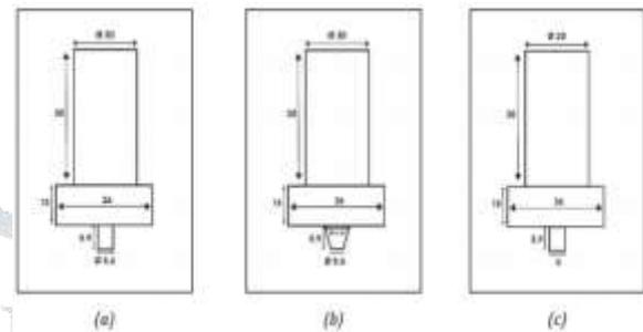
Figure 4: (a) Cylindrical pin tool; (b) Tapered pin tool; (c) Square pin tool [13]
