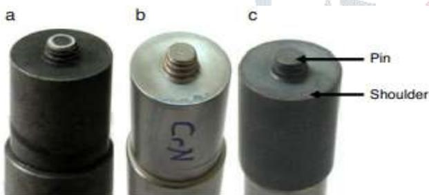
Figure 3: FSW coated tool [10]
