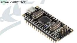
Summary Microcontroller ATmega328 Operating Voltage 5V Input Voltage (recommended) 7-12V
