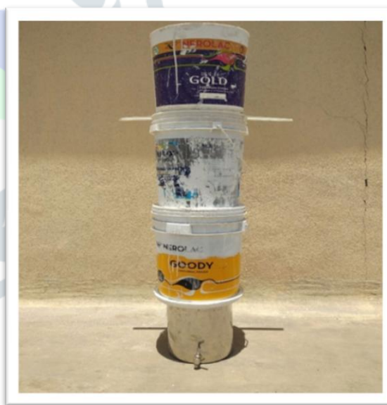
Fig 3 :- integrated grey water treatment plant
