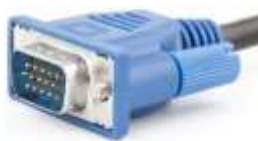
Figure 1.2 VGA cable with DE-15 male connector
