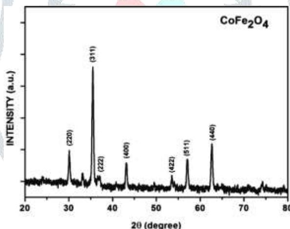
Fig. 1 X-ray diffraction pattern of spinel cobalt ferrite nanoparticles
