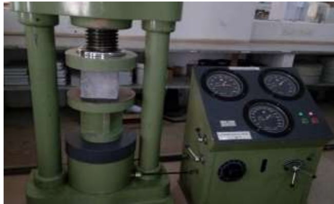
Fig 1: Compressive strength testing of concrete
