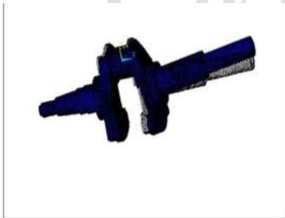
Fig- 3.3 Deformation of crankshaft
