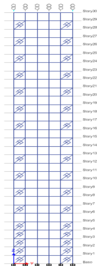
Fig 2 Building with Viscous damper
