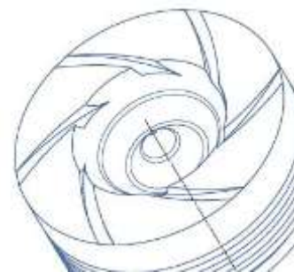
Fig.4.5 Schematic representation of SSCV piston
