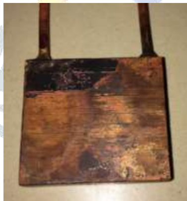
“Fig.2” Copper Plate (40 x 40 mm) with Thermocouple Connection
