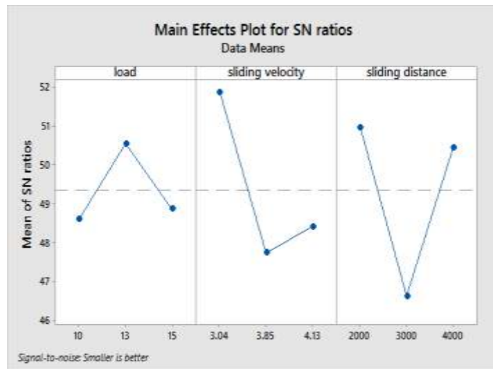
Fig. 8 S/N ratio of LM9 alloy-Wear
