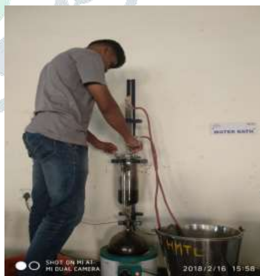
Figure 5: Road Samples Collected Using Core Cutter Figure 6: Soxhlet Extractor
