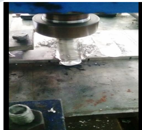
Fig 5.2 Milling machine with loaded work piece Basically no defect was found in FSW. No defects like crack, tunnel, pin hole, piping and worm were
