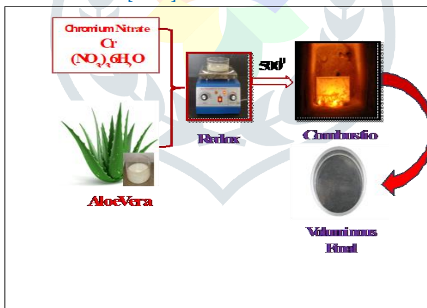
Fig 1 Flow Chart for Preparation of \text{Cr}_2\text{O}_3 NPs
