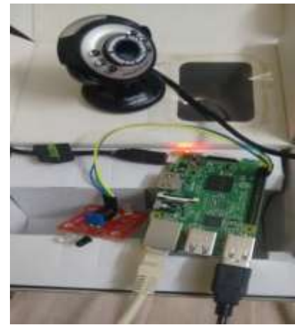
Fig7: ARM board with interfacing of sensor UVC driver camera and display unit
