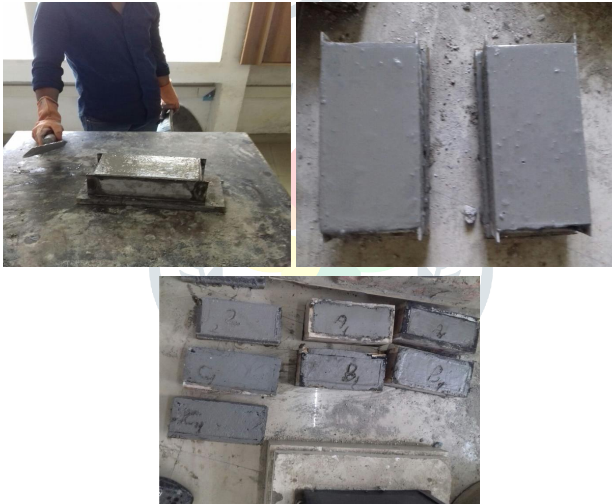
Figure 4.1: Casting of the bricks
