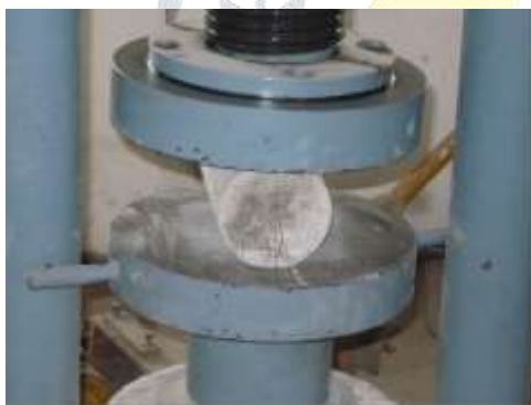
Fig 4.2 Failure of Cylinder Specimen
