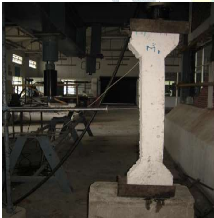
Fig 5.1 Experimental Test Setup for Short Columns
