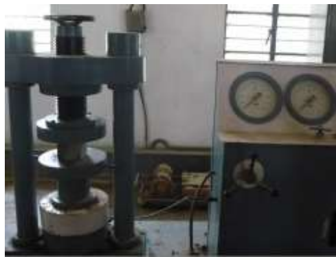
Fig 4.1 Testing of cubes in CTM
