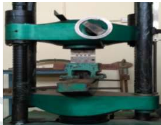
Figure 2: Compaction of powder by using UTM
