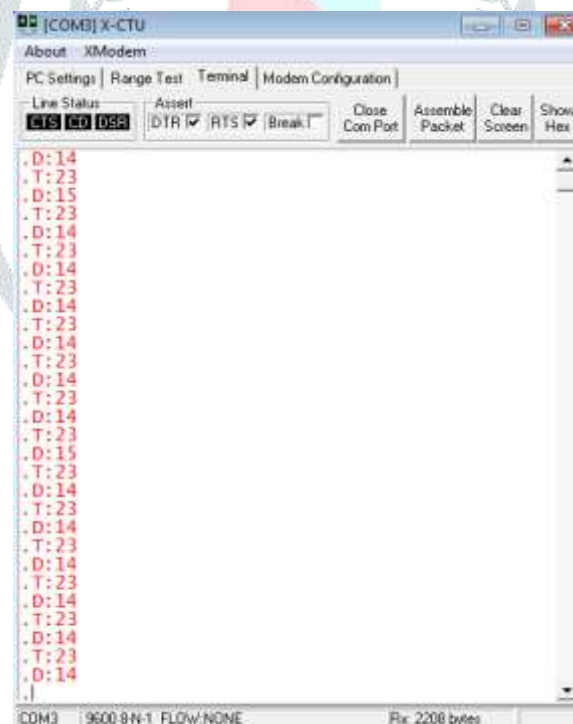
Fig.4 Serial monitoring of the object distance and temperature
