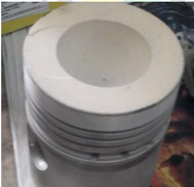
Fig. 3. Yitriya stabilized Zirconia coated piston
