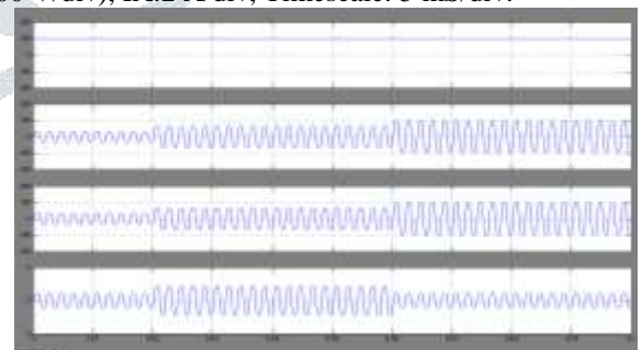
Figure 8: Pole, Phase, capacitor voltages along with current for 40-Hz operation of the converter. VAC1:(50 V/div),VAO: Pole voltage(100 V/div),VAN: Phase Voltage (100 V/div), VAC4: (10 V/div),VAC3: (10 V/div),VAC2: (100 V/div), IA:2 A/div, Timescale: 5 mS/div.
