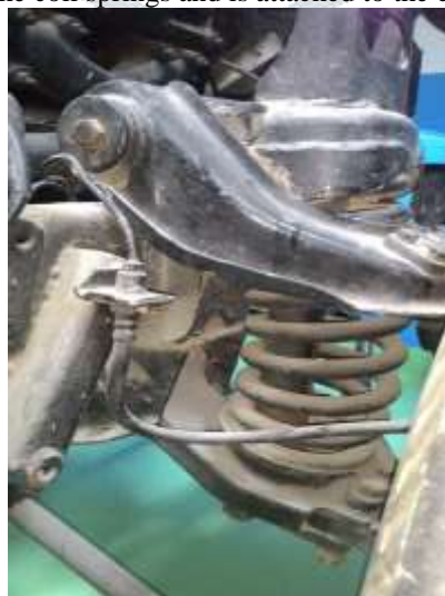
Fig. 1 Present double wishbone suspension system.
