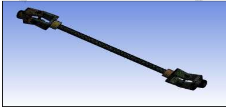
Fig.1-Finite Element model of steel/GFRP Propeller Shaft
