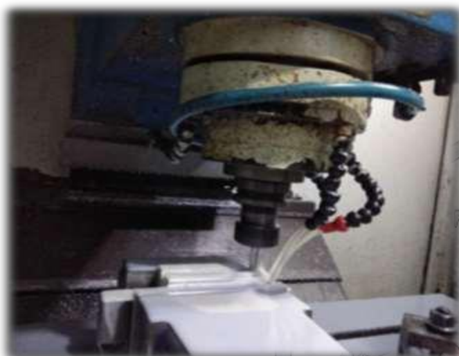
Fig5.1 Machining of 5083 Aluminum alloy with cutting fluid
