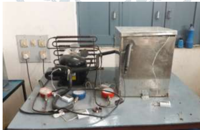
Fig .2 VCRS with new designed condenser
