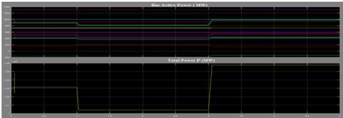
Figure 18. Active power (P) of all buses and sum of total active power at the buses.
