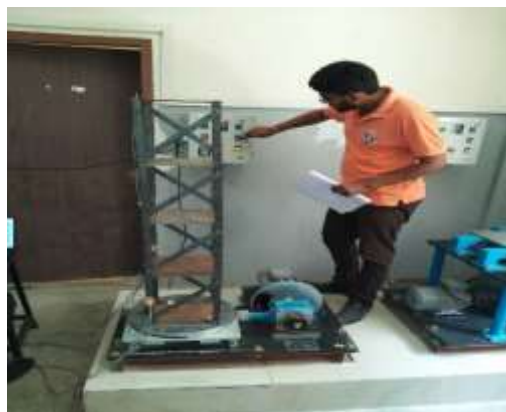
Fig 3.5 Shake table test with bracing
