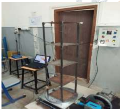
Fig 3.4 Shake table test without bracing
