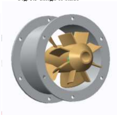
Fig. 3.5 design of impeller and casing mesh
